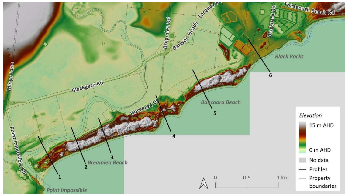
Figure 12. Elevation (LiDAR) across the Breamlea and Bancoora area. Source: 2020-21 Golden Plains Area LiDAR. Profiles shown in Figure 13.
